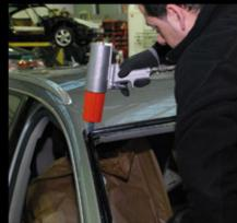
There are two versions: the 3900 Plus for sealants in cartridges and the 3900 Plus M for sealants in sausages. Both versions include a trigger with discharge valve, which guarantees a great precision and control.
