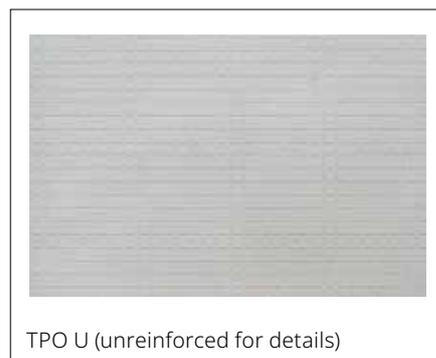
KÖSTER TPO 2.0 U is an unreinforced sheet for the KÖSTER TPO roofing and waterproofing membranes for the manual production of corners, gullies, flanges, and corner protection.
