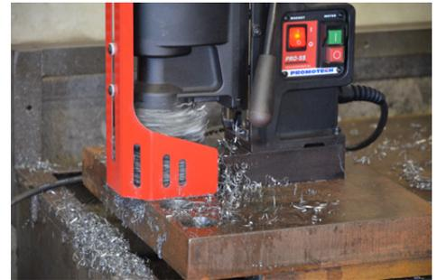
Milling capacity up to 55 mm (2.17")
