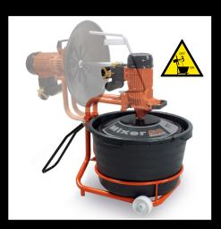
An automatic safety switch prevents the motor start when the mixing head is completety raised up.
