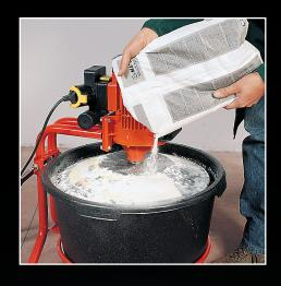
The material must be poured on the black plastic protection.
