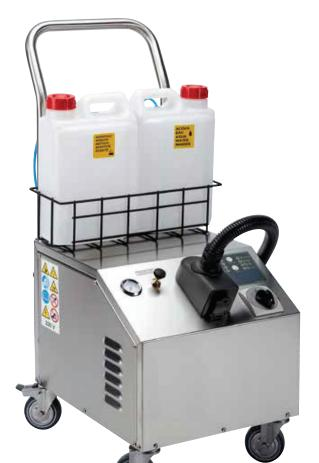
• Satured steam at 9 bar at 175°C temperature • Steam gun with low tension control • Made of AISI 304 stainless steel • Boiler 3,3 kW S/S AISI 304. Thickness 25/10 • Heating and activation time required: 7 min. • Steam regulation • Discharge valve • Pressure gauge • Device for using chemicals and detergents mixed with steam • The boiler can be refilled from the tank provided (continuous duty) • Pivoting wheels with brakes, suitable for use in food processing areas.
