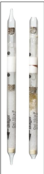
Standard Measuring Range: 0.1 to 1 mg/m<sup>3</sup>
