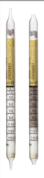
Standard Measuring Range: 100 to 700 / 5 to 150 ppm Number of Strokes (n) : 2 Time for Measurement : app. 50 s / app. 4 min Standard Deviation :  $\pm$  10 to 15 %
