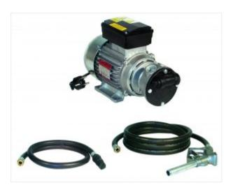
For oil transfer - 40 lt/min. Self-priming, rotary, vane pump, with protection class IP55 and by-pass valve. For diesel and oil, with rubber exit hose (4 mt), aluminium gun, rubber tail pipe with filter. Max pressure 2-3 bar. Maximum output 70 lt/min.
