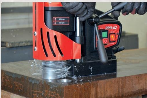
Milling capacity up to 65 mm (2-9/16")
