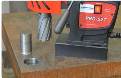
Milling capacity up to 50 mm (2")
