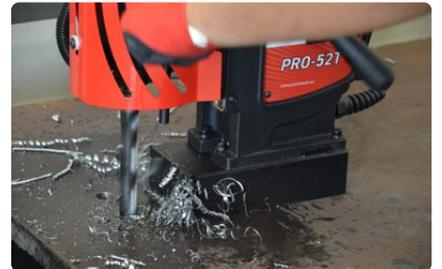
Drilling capacity up to 23 mm (7/8")
