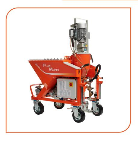
Single-phase (230 V) continuous mixing pump, ideal for spraying pre-mixed surface coatings containing lime, cement, finishing compounds, fillers, coloured compounds, adhesives, screeds, etc. and any product compatible with mechanical spraying.
